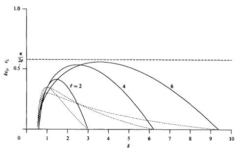
FIGURE 3. Sheared-disturbance stability problem: the imaginary part of the phase speed Im  $(c_2)$  (dotted line) and growth rate  $\kappa \operatorname{Im}(c_2)$  (solid line), as predicted by (3.20), plotted against wavenumber  $\kappa$ . The cases  $\hat{\tau} = 2$ , 4, 6 are shown. The predicted large- $\tau$  value of Im  $(c_2)$ , which is  $\pi/2e$ , is marked by a dashed line for comparison.
