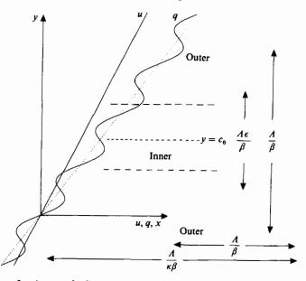
FIGURE 2. Regions for the matched-asymptotic analysis, together with the basic flow and basic-state absolute-vorticity profiles. The inner region is described by the coordinate Y and the outer region by the two coordinates y and  $Y(=y/\epsilon)$ . For the calculation presented in §3 the wavelength of the sheared disturbance  $\Lambda/\beta\kappa$  is taken to be much larger than  $\Lambda/\beta$ .
