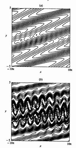
FIGURE 6. Contours of absolute vorticity in experiment (iii) at (a) t = 11 and (b) 19. The contour interval is 0.5.
